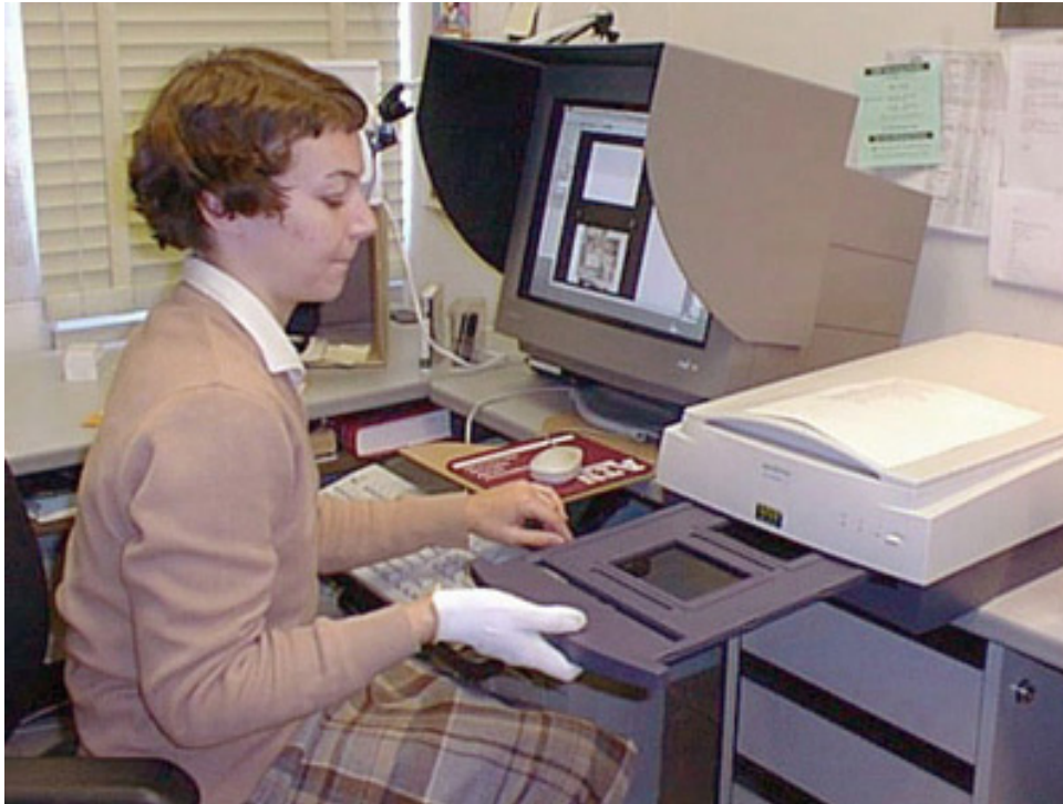
Figure 2. A project assistant working with 4x5-inch transparencies on the Microtek Scanmaker V.
