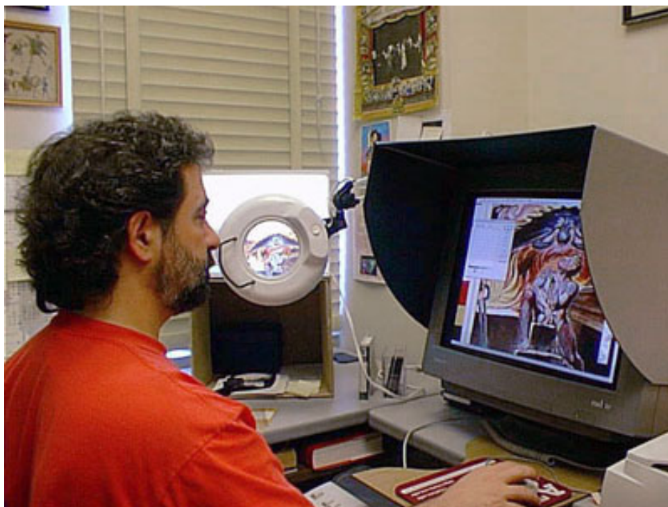
Figure 4. Color-correcting a 300-dpi TIFF image in Photoshop. Note the color bar on the TIFF, the monitor hood, and the 4x5-inch transparency visible through the magnifying glass on the lightbox.
